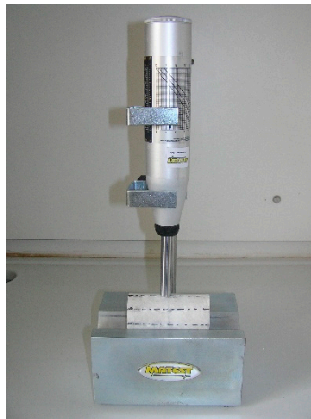
Figure 4. The Schmidt hammer rebound test.
