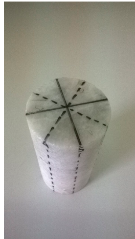
Figure 3. Straight parallel lines drawn along the longitudinal axis of each specimen.
