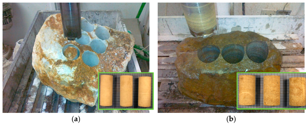
Figure 1. Core specimens of (a) marble and (b) metasandstone.
